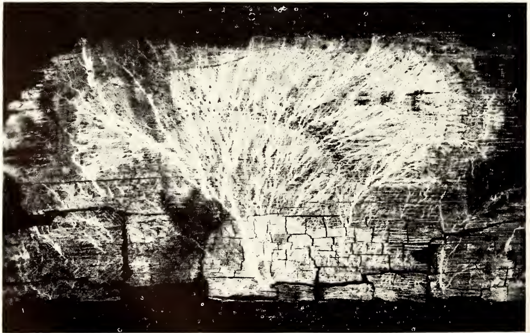
FIGURE 2-94.—Mycelium on oak and the characteristic cracking of typical brown rot.
